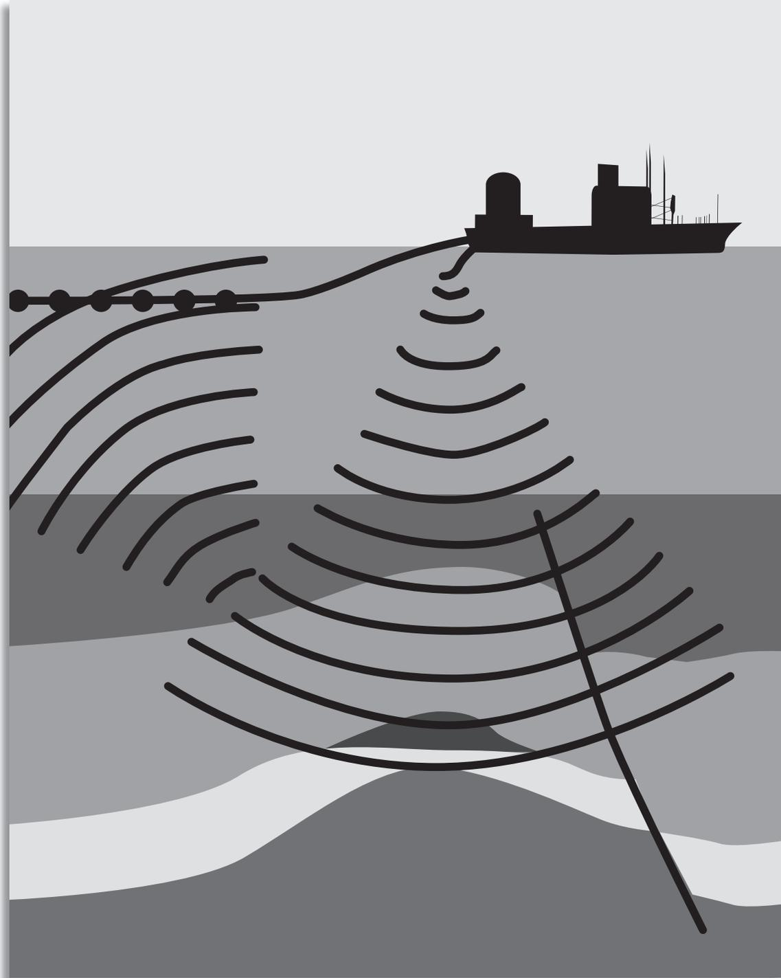
widely spaced lines are used for reconnaissance work and shorter, more closely spaced lines are used to define actual drilling targets.
